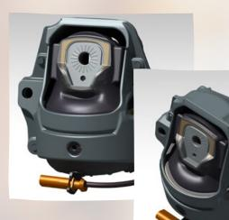
The electronic hydro-mount represents an innovative and enhanced version of the conventional hydraulic mounts. This type of hydraulic mounts is controlled by the vehicle ECU, through an actuator, the mount's dampening capacity can be altered depending on the vibration caused by the engine.
